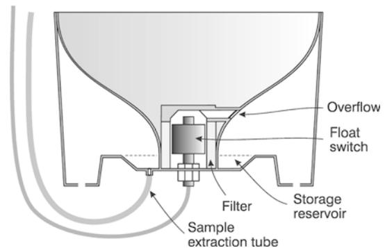
**Fig. 5** A schematic of the wetting front detector showing the filter, cavity, float switch and overflow reservoir for collection of soil solution
